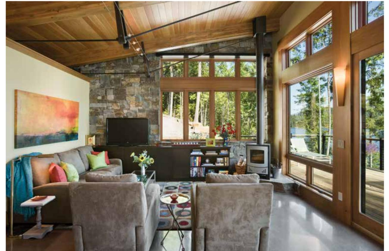
Because of their durability and water resistance, concrete floors were a natural choice for the entire cabin, and the slab-on-grade construction keeps them cool even on the hottest days. Schlauch Bottcher Construction ground down the concrete so that the aggregate is exposed, a detail that ties the floor further to the cabin’s lakefront setting.
